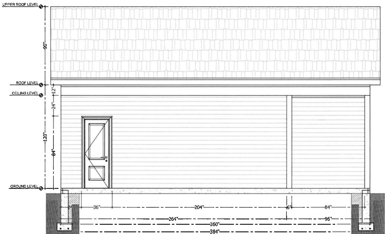
Right Elevation Grade Scale: 1/8"=1'-0"
